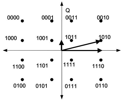
Figure 2. 16-QAM Signal Constellation showing IQ decomposition
