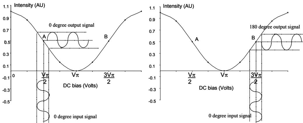
Figure 4. MZM Bias Switching to Achieve Bi-Phase Modulation
