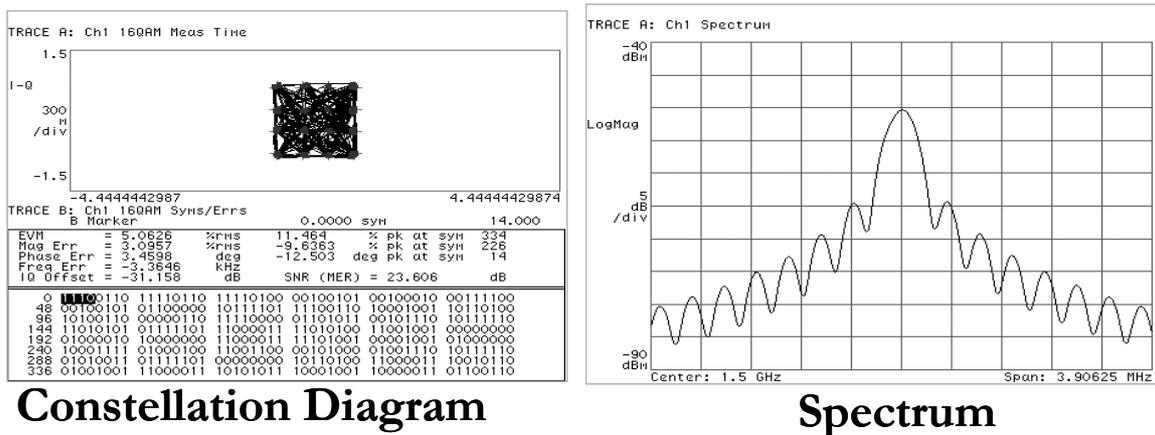
Figure 7. 16-QAM Constellation Diagram and Spectrum at  $f_c = 1.5$  GHz
