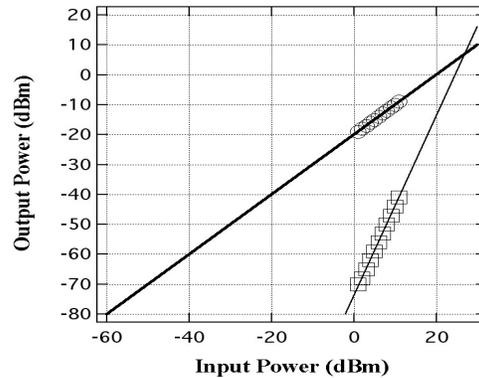
Fig. 4. Linear extrapolation of fundamental (circles) and third order distortion (boxes) output RF power as a function of input RF power. Data displayed yield  $OIP3 = 7$  dBm for  $I_{DC} = 10$  mA at 10.4 GHz. The noise floor is at  $-148$  dBm for a 1 Hz bandwidth.
