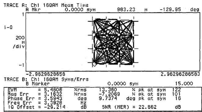
Fig. 3. Experimentally measured 16-QAM signal constellation diagram.
