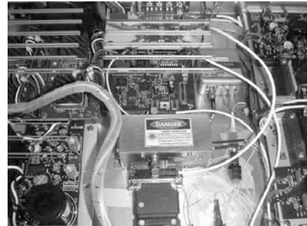
Figure 5. Microchip laser source
