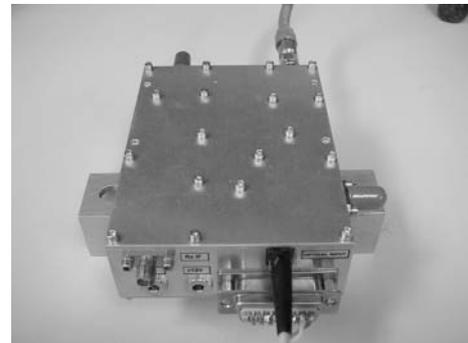
Figure 6. Basestation Photograph – the size is 4.0" x 3.0" x 1.25"
