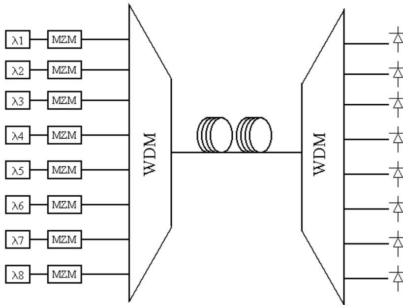
Figure 1. Eight channel WDM RF delay line.
